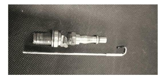
The tool is screwed into number one cylinder and by rotating the engine the compression stoke can be found by feeling the pressure increase with one's thumb on the connector or by taping a balloon onto it and watching the inflation and deflation.
