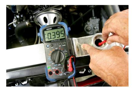
A little-known cooling system condition diagnostic trick is to measure the acidity level of the antifreeze by reading the voltage of the coolant. No kidding. This is a simple test using either a digital voltmeter or an old school analogue voltmeter. With an analogue meter, set it to read to measure in the under 1-volt scale.
